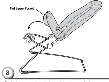
• Fit the lower pocket on the back of the pad onto the footrest.
